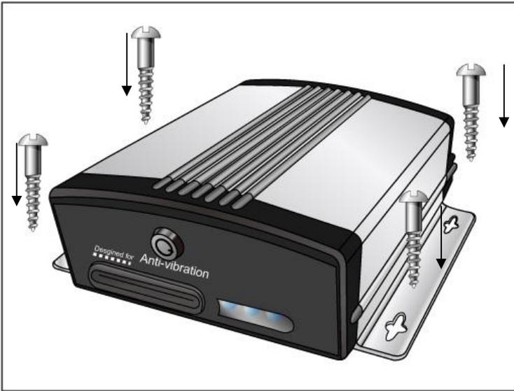
Fasten four screws into the holes
