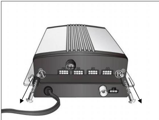
Loosen the screws in (A) and (B)
