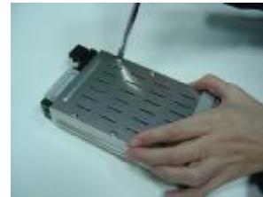
Step 4 Loose all screws on the Cartridge
