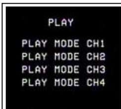
When changing the channels, users can either press the buttons "1- 4" on the front panel or enter the "PLAY MODE" menu for displaying.
