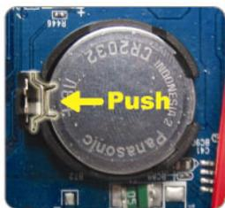
Step5: Get a new battery with the side of “CR2032” facing up, and install it to the mainboard.
