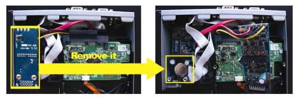
Step4: Push the release as indicated below to remove the battery.
