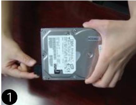
Connect the connector with the HDD.
