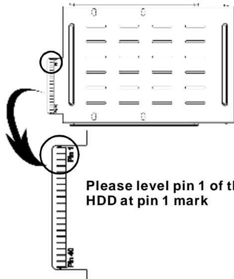
Please level pin 1 of the HDD at pin 1 mark
