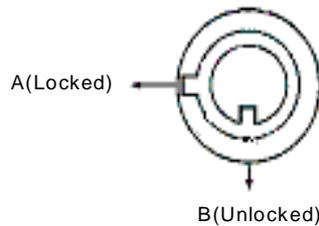
Lock the cabinet by turning the key clockwise. Close the cap.
