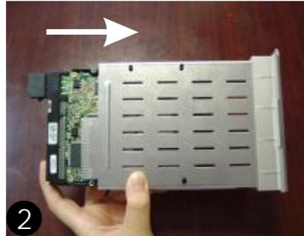
Put the HDD into the HDD cartridge. Please notice the bottom side is power side.
