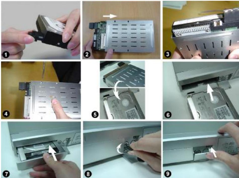
Step 1 Connect the connector with the HDD (refer to Picture 1).
