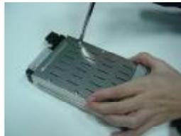
Step 4 Loosen all screws on the Cartridge
