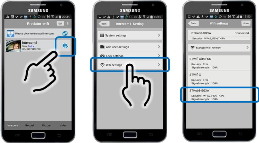
Check that the network which it is connected to is showing at least 20% strength. If it is not connecting, or is lower than 20%, then corrective action must be taken at this stage. Suggestions are as follows..
