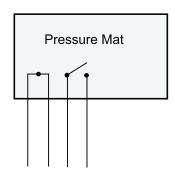
In a 4 wire configuration the two wires on the far left are the tamper loop. These are only needed when connecting to an alarm control panel.
